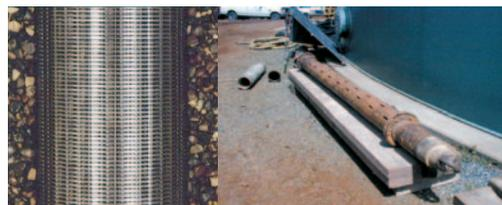
**Figure 7.** Example of gravel pack around a wire wrap screen (left) and picture of swab/air lift tool used to develop a well (right).
