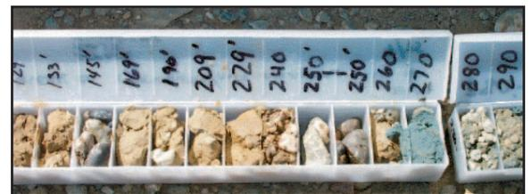
Figure 4. Sample drill cuttings collected and separated by depth. Note the change in color and gravel content among the samples.
