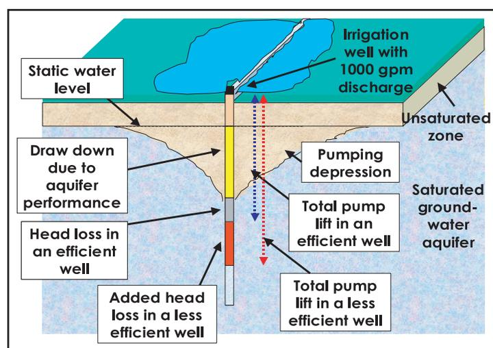
Figure 1. Schematic showing concept of well efficiency.
