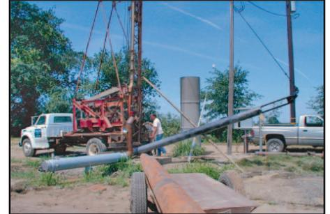
Figure 2. Cable tool drill rig. Note, small rig and no drilling fluid or pit needed.
