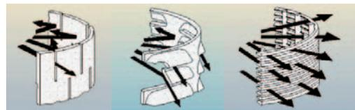
**Figure 6.** Three types of well screen. Mill slot (left - 2 to 3 % open area), Louver screen (center - 8 to 50 % open area), and Wire Wrap screen (right - 30 to 50 % open area).
