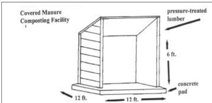
Proper storage of horse manure for composting can be handled in several ways and storage structures are sized based on the number of horses. It may be as simple as a concrete pad with concrete or wooden walls that may or may not have a roof. Bins with wooden floors can also be constructed. With a large number
